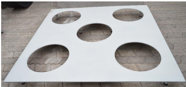
Heavy-duty floor panel with height-adjustable feet for leveling uneven surfaces.
